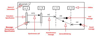
Figure 1: Example Sequence Diagram
