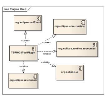
Figure 3.6: Plug-in Dependencies of the TERMOS Tool
