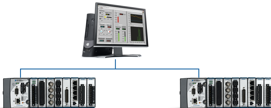
Figure 5.1. The simplest method of adding another CompactRIO system as Ethernet I/O involves connecting two CompactRIO systems to the same network.
