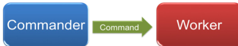
Figure 3.15. A command-based architecture provides a mechanism to send commands between parallel tasks.
