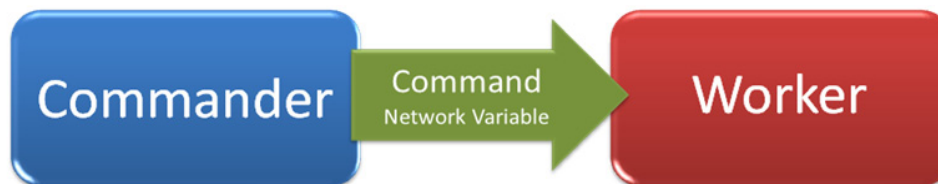
Figure 4.12. Simple Command Architecture Using Network Variables
