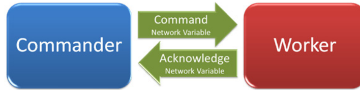
Figure 4.31. Simplified Acknowledged Command Architecture Using Network Variables
