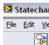
Figure 2.34. Click on the icon on the upper left corner to generate code for the statechart using LabVIEW.
