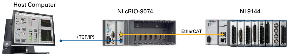
Figure 5.9. To configure the deterministic Ethernet system, connect Port 1 of the cRIO-9074 to the host computer and connect Port 2 to the NI 9144.
