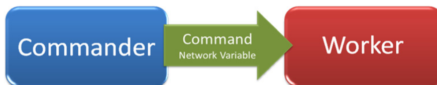
Figure 7.2. Simple Command Architecture Using Network Variables
