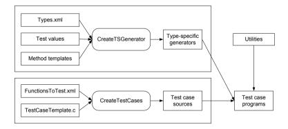
Figure 2. Architecture of the testing framework
